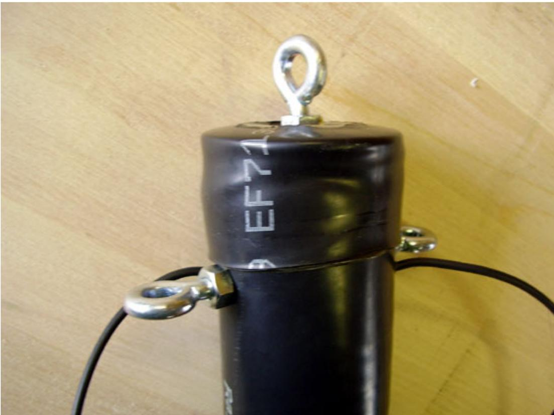
*Antenna Wire attachment and connections*
